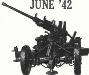
Received assignment to produce the famous Bofors 40 mm. automatic field gun. Capable of firing 120 rounds a minute, this is the largest automatic weapon used by the Allied Nations. It is "effective against land, air or water targets."
